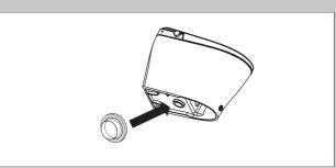
2. Fit the sealing flange snugly into the toilet's drain 3. Based on the previously drawn contour line, set the ceramic toilet onto the outlined position.
